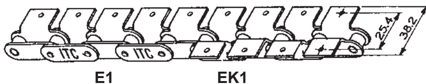
ATTACCO MAGLIA INTERNA INNER PLATE ATTACHMENT
