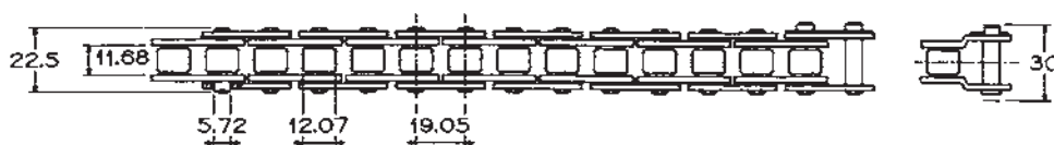
ATTACCO MAGLIA INTERNA INNER PLATE ATTACHMENT
